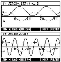
Unlike the **SYMB** mode where the *b* coefficient goes up or down in steps of 0.1, the increments in **PLOT** mode are not regular but are chosen to be 'nice' fractions of  $\pi$ . The slight difference in results is most easily seen by simply experimenting.
