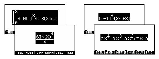
Notice the lack of a '+c' indefinite constant in the integration result. Here, this is because we are using the definite integral (see page 81 and the page following). A better alternative is to use the **INTVX** function as shown below, even though it still does not add the '+c'. See the page after this for information on using functions in the CAS.
