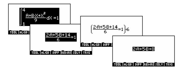
As can be seen above, the initial integration gives an equation involving a fraction. This can be simplified by multiplying both sides by 6, highlighting the entire equation first. Notice that when the final simplification is equal to zero, the calculator does not bother to include the '=0'.
