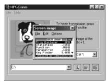
your calculator screen will appear. If it doesn't then check that you have fresh batteries in the calculator and investigate the use of a different serial port.
