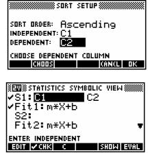
The S1:, S2: ... refer to data sets 1, 2... This allows you to display more than one set of bivariate data by specifying the columns for each set. Columns can be used in more than one set. Note that a 'C' screen key is provided for your convenience.
