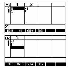
Step 3. Change into the **HOME** view and enter the calculation  $M1^{-1}*M2$ . The result is the (x,y) coordinate of the solution.
