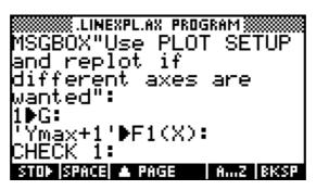
A message is first given to the user of how to proceed if they want to use different axes. The flag value of **G** is then set to 1 so that the next program can tell that the axes are ready to use. The function is also re-entered in case the user has changed the **SYMB** view. Users have a habit of changing things so try to allow for this in your programs.
