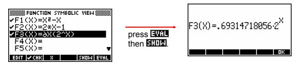
As you can see the calculator's algebraic abilities do not extend to differentiating  $f(x) = 2^x$  as  $f'(x) = \ln(2) \cdot 2^x$ , but at least it is numerically correct.
