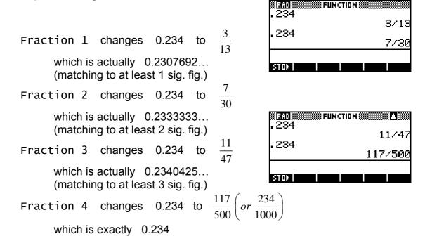
Essentially, the value of 'n' in 'Fraction n' affects the degree of precision used in converting the decimal to a fraction. As was said earlier, the calculator will use the first fraction it finds in its process of approximation which matches the decimal to that number of significant digits.
