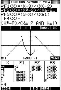
By dividing by the domain expression we are effectively dividing by 1 inside the range (no effect) or dividing by zero outside the domain, making the function undefined. Since undefined values are not graphed, this produces the desired effect.
