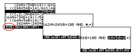
We can then finish off the LINSOLVE command by pressing right arrow to move to the second parameter position and then entering "A AND B". At that point we can press ENTER to obtain the values of A and B.
