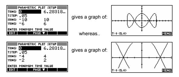
Notice that in both cases, **TRACE** is on and shows the T value, followed by an ordered pair giving (X,Y). Unlike XRng & YRng, the effect of TRng is to decide how much of the graph is drawn at all, not how much is displayed of the total picture.
