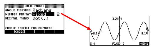
This setting also applies to the appearance of equations and results displayed using the **SHOW** command.
