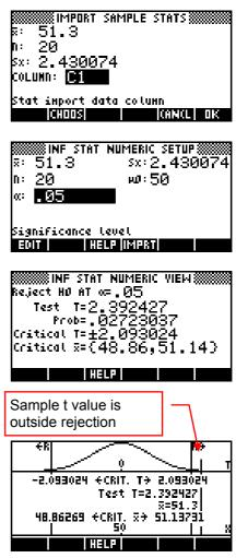
The test value for the Student-t and the sample mean are listed in the middle of the screen and the rough position of these values is shown by a vertical line in both the upper and lower diagrams. The regions for rejection of the null hypotheses are shown at the very top of the screen by the ' $\leftarrow$  R' and 'R $\rightarrow$ '.
