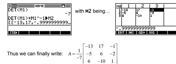
An alternative to this is to change into *Fraction* 6 numeric format in the **MODES** view. This will give a matrix of fractional values which can be seen more clearly using **ETITA**.
