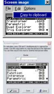
A variation of this capture process is useful if you want to retain the image on your calculator. Pressing **ON+PLOT** stores the image into graphics object G0. This can then be pasted into a sketch using the VARS menu. From the **Sketch** view, press **VARS** and then
