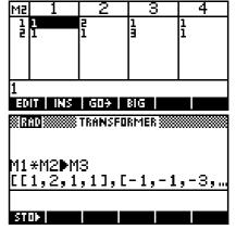
The result is a triangle with corners at (1,1), (2,1) and (1,3), along with its image after reflection in the x axis.
