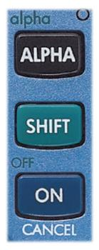
The SHIFT key gives you the second function for each key. In the case of the COS key, the second function is ACOS, sometimes referred to as arc-cos or cos<sup>-1</sup> or inverse cos. Most keys have these second functions that are obtained via the SHIFT key.
