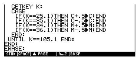
A **CASE** statement is then used to check for the use of the arrow keys. Notice the lack of colons (:) after each **END** in the **CASE** statement.
