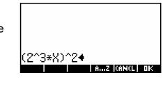
If you want to delete the entire expression then the simplest method is to press **ON** and exit the CAS and then re-enter it with a blank screen. Alternatively you can highlight part or all of the expression and then press **SHIFT ALPHA CLEAR**. The highlighted section will be cleared.
