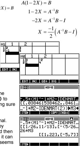
Finally use the **HOME** view to calculate the answer, using the function **IDENMAT(2)** to produce a 2x2 identity matrix, and making sure to store the result into **M3**.
