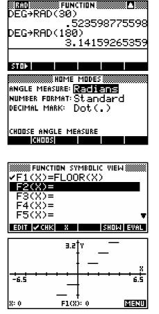
function then you will need to use the **PLOT SETUP** view to turn off CONNECT first, since the graph is supposed to be a discontinuous step function. The result with CONNECT turned on is not good.
