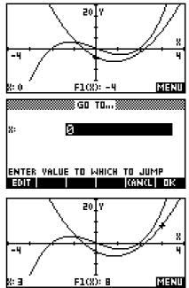
A very nice feature of the **E** key is that it will jump to values which are not on the current screen, or which would be inaccessible for the current scale.
