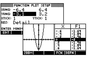
Using -3.2 to 3.2 is even better since it makes the graph 'square' again, with both axes proportional. Another good choice of scale for the *Plot-Table* view is -8 to 8, giving table values of 0.25. Basically any power of 2 is a good choice. Again, adding or subtracting a
