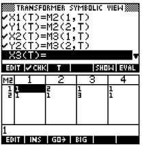
substitute the actual values from matrix M2 then these points become (1,1), (2,1), (3,1) and (1,1), which give the shape when plotted. The repetition of the first point is to ensure that the line forming the triangle is closed by connecting back to its starting point. Obviously X2 and Y2 perform the same function with matrix M3.
