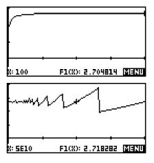
This apparent instability is caused by the internal rounding of the calculator. It works to
