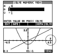
When you select **B** by highlighting it, the calculator substitutes the supplied values into all other variables except **B** and graphs the left and right sides of the equation as two separate graphs. This may not always be obvious because the substitution may produce graphs which aren't visible on the default scale.
