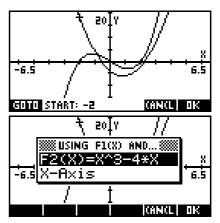
We now need to choose the end point. This time do it by tracing with right arrow to move the cursor. As you do the area will be shaded by the calculator. The current position is shown at the bottom of the screen. When you reach the end point you are looking for, press the **OK** key and the area will be calculated as before. This is shown right.
