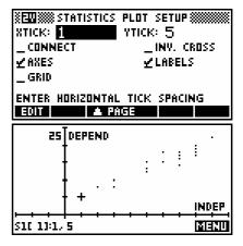
point in data set S1 whose value is (1,5). Using the left/right arrow keys you can move this cross through the data set with the values being reported at the bottom of the screen.
