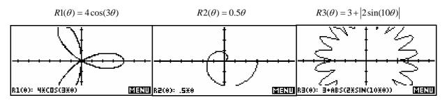
The **PLOT SETUP** view shows that ranges must be specified not only for X and Y but for  $\theta$ . The values set for XRange and YRange control the length of the axes. The movement of the cursor follows the increments set for  $\theta$  in  $\theta$ Step regardless of the resulting X and Y positions.
