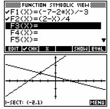
It is worth noting that although the point of intersection is on the screen here, this is not necessary. The **EXI** Intersection tool will work even if neither line is visible on the currently set axes.
