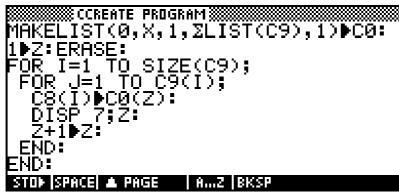
We'll now use this program to expand the frequency table I built earlier. The first thing we need to do is to move columns C1 and C2 to **C8** and **C9**. Rather than re-typing, this can be done in the HOME view as shown.
