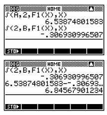
can use the accurate values you stored in Step 4. It needs to be done in two parts and added (subtracted actually to reverse the sign of the negative part). This is shown right, with the **COPP** key having been used to add the values.
