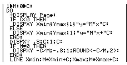
The first line assigns initial values to the variables **M** (gradient) and **C** (y-intercept). The **DO...UNTIL** loop which follows (partly in the next section of code) loops through the code within it until the **ENTER** key is pressed.
