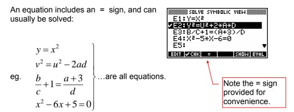
An expression, on the other hand, does not contain an = sign. It can be evaluated or rearranged but not solved. When you enter an expression into the Solve aplet it internally puts an " = 0" onto the end so as to convert it into an equation which can be solved.
