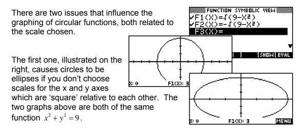
The simplest way to deal with this is to use scales which are multiples of the default scales. For example by using  $-13 \le x \le 13$  and  $-6.2 \le y \le 6.4$  (scale factor 2). You can also use the 'Square' option on the **ZOOM** menu. This adjusts the *y* axis so that it is 'square' relative to the *x* axis chosen.
